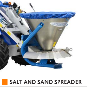
SALT AND SAND SPREADER
